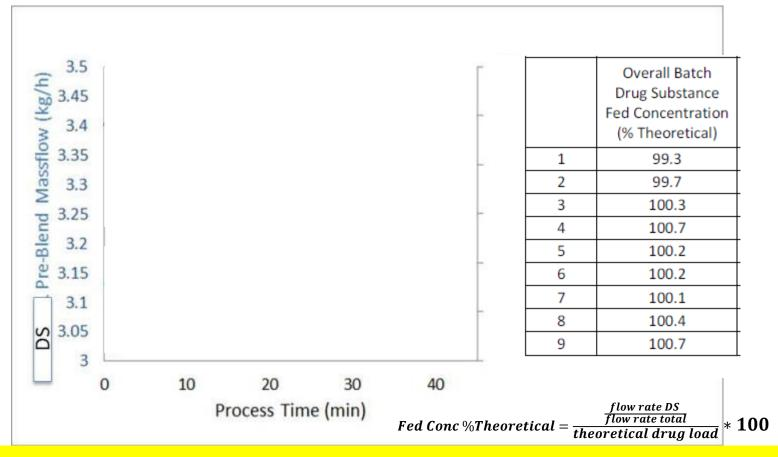
Feeder ratio mode addresses both common cause variation and deviation from target All feeders are driven in the same direction as the DS feeder variation Ratio mode is in addition to individual Feeder controls (Level 1 control)
