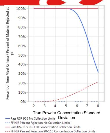
Operating characteristic (OC) curves demonstrate that using in-process NIR for product collection control ensures content uniformity requirements will be met
