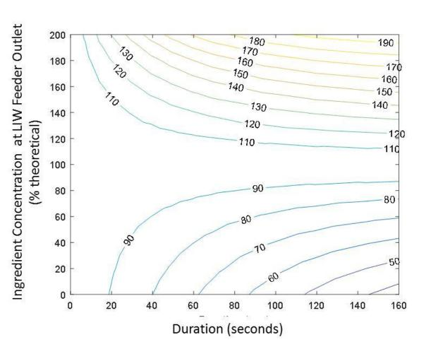
Simulations using flow sheet model generated "funnel plots"
